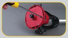
Unscrew Phillips screws that hold base plate to motor housing without removing base plate.
